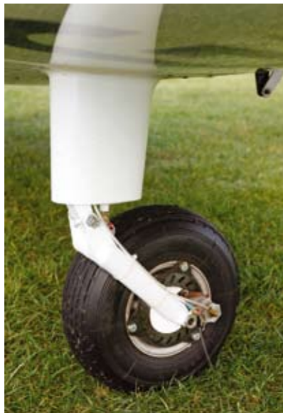
Far Left: The nosewheel strut is rugged, while elegant trailing-link units carry the mainwheels. Note that the discs are drilled.
