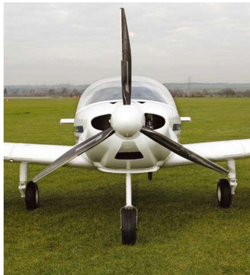
Left: The propeller is a ground adjustable three-blade DUC 'Swirl'. Interestingly, the blades twist under aerodynamic loads. This essentially changes the pitch, providing some of the advantages of a CS prop without the complexity.
