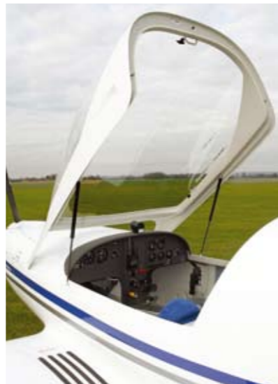
Right: The canopy is well supported by gas struts.
