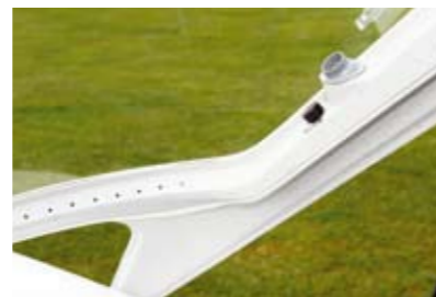
Right: There are separate fresh air nozzles for each pilot built into the canopy frame.
