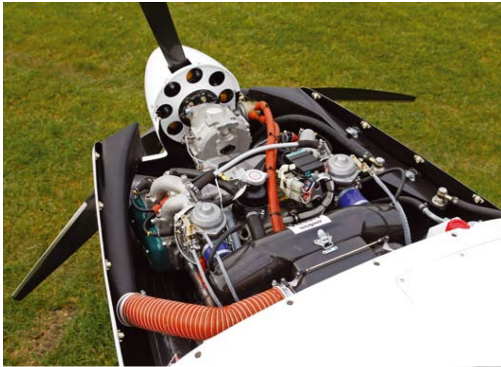
Above: Access to the engine is good, as the top cowling is secured by 'Dzus' fasteners and can be quickly removed.
